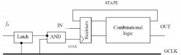
Figure2. Schematic diagram of gated clock design
