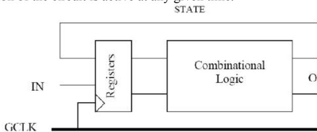
Figure1. Single clock, flip-flop based FSM.
