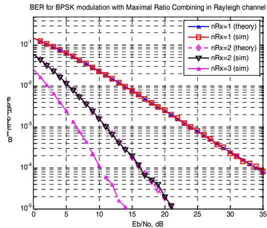
“Figure 5: BER for Maximal Ratio Combining”
