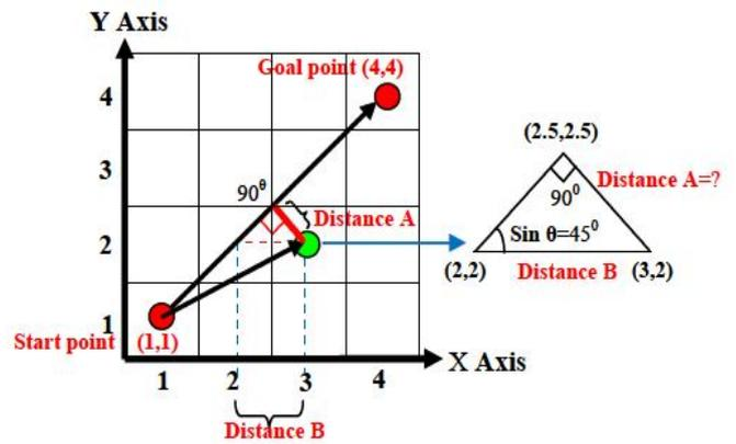
$$\begin{aligned} \text{Distance A} &= \sin \theta * \text{Distance B} \\ &= \sin \theta * \sqrt{(y_2 - y_1)^2 + (x_2 - x_1)^2} \\ &= \sin 45^\circ * \sqrt{(2 - 1)^2 + (3 - 1)^2} \\ &= 0.7071 * 1 \\ &= 0.7071 \end{aligned}$$
