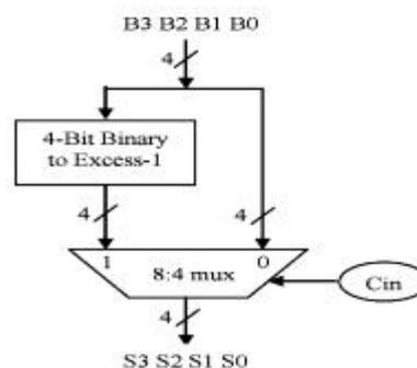
Fig. 3. 4-b BEC with 8:4 mux
