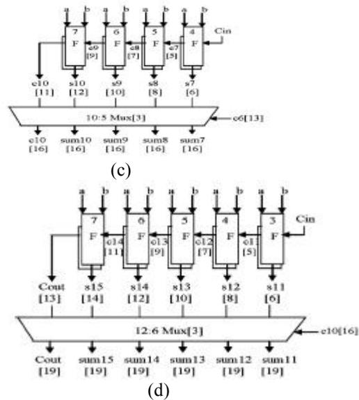
Fig. 5. Delay and area evaluation of regular SQRT CSLA: (a) group2, (b) group3, (c) group4, and (d) group5. F is a Full Adder
