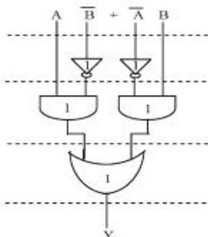
Figure I. Delay and area evaluation of an XOR gate
