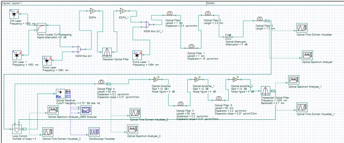
Fig1. Simulated circuit for generation and analysis purpose
