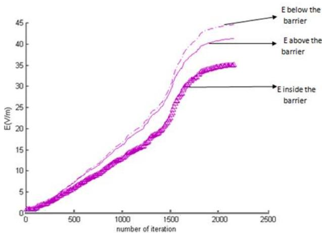
Fig 7 Electrical Field above, inside and below the barrier
