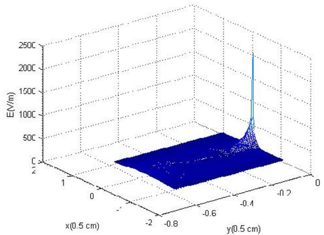
(b) Field just before breakdown (10 mm Barrier Width)
