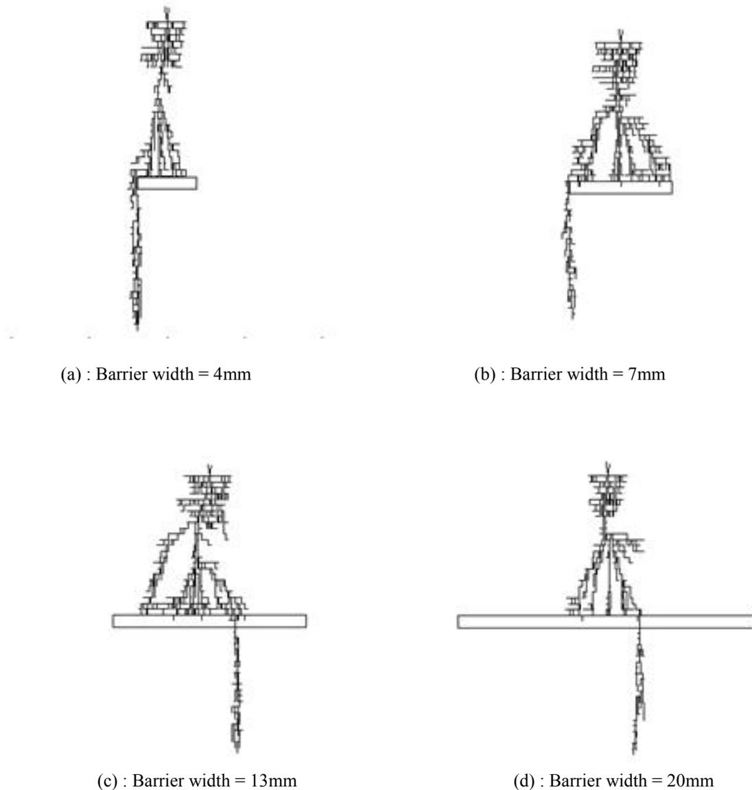
Fig.2 Tree Progression for different barrier width
