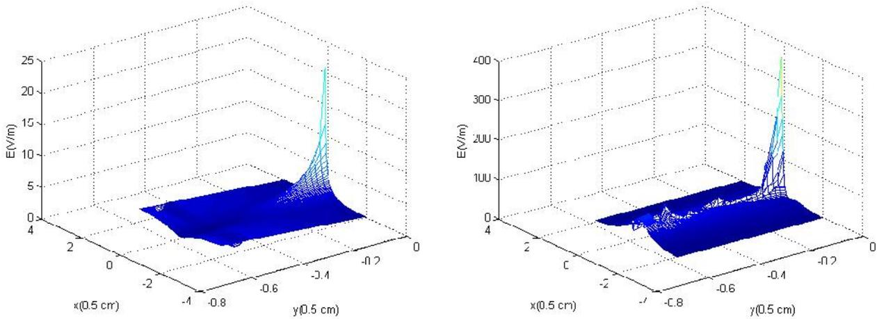
(a) Field before tree inception(20 mm Barrier Width) (b) Field just before breakdown (20 mm Barrier Width)
