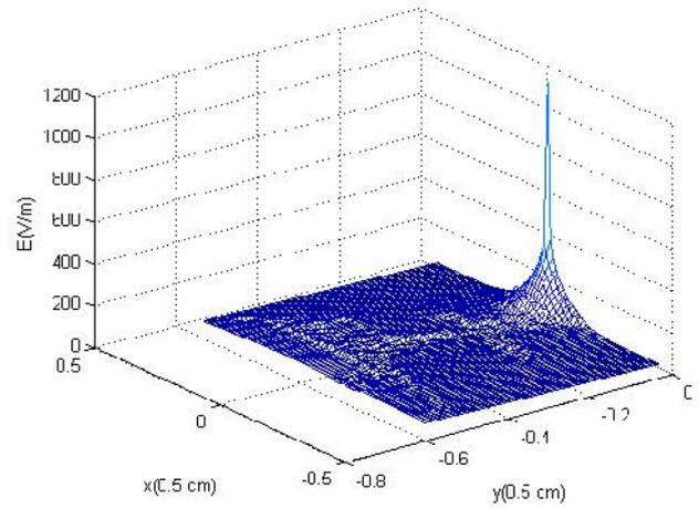
(b) Field just before breakdown (4 mm Barrier Width)
