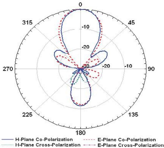
Fig. 9 Radiation patterns at 62.5 GHz
