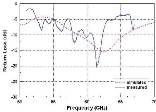
Fig. 7 |S11| for the antenna array
