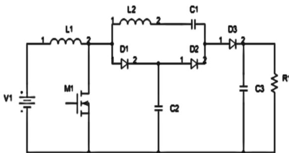
Fig 2. Voltage Multiplier Cell
