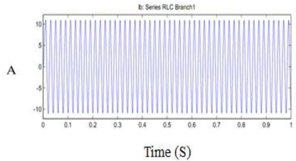
Fig 7. Inverter current of 10 Apk-pk
