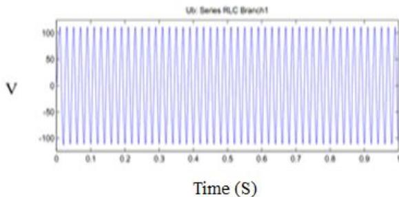
Fig 6. Inverter voltage of 100 V pk-pk
