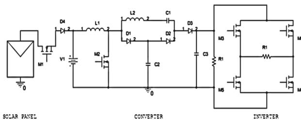
Fig 8. An integrated inverter with solar charge controller
