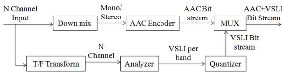
Fig 9 .Schematic diagram of VSLI-based SAC encoder [7]
