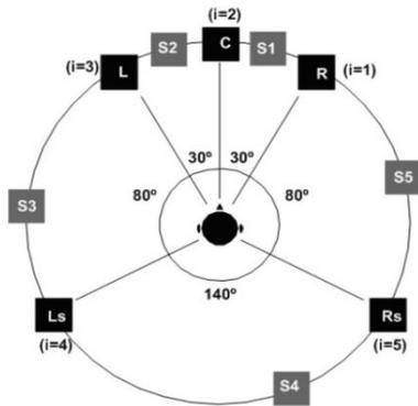
Fig 8 .Playback speaker layout of VSLI Method [7]
