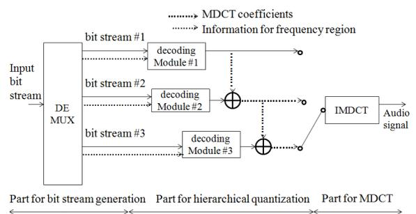
Fig 5 .Structure of Scalable Decoder [4]
