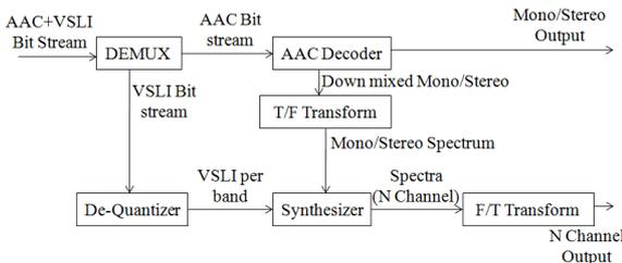
Fig 10 .Schematic diagram of VSLI-based SAC decoder [7]
