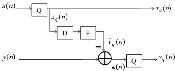
Fig 2(a) .Encoder block diagram of AICP [3]
