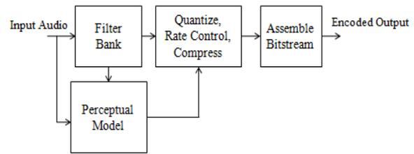
Fig 1 .Block Diagram of Perceptual Audio Coder (PAC) [2]
