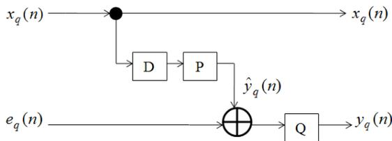
Fig 2 (b) .Decoder Block diagram of AICP [3]
