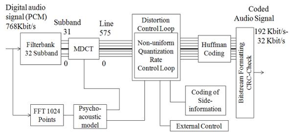
Fig 7 .Block diagram of MP3 Encoder[6]
