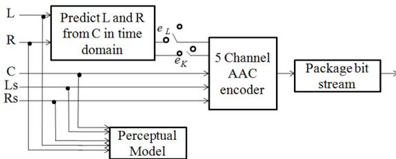
Fig 6 .Prediction-incorporated AAC coder[5]
