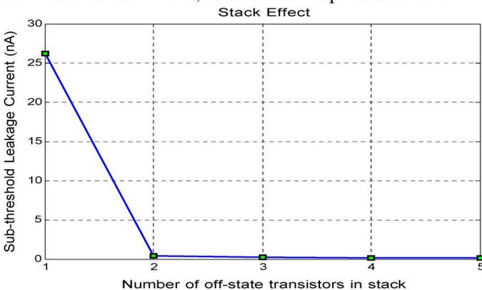
Fig. 7. Leakage current decrease with an increasing number of off transistors in stack (where  $V_{DD} = 0.9$  V is applied to 32-nm n-MOSFETs with 0.9-nm oxide thickness and  $W/L = 128$  nm/32 nm).
