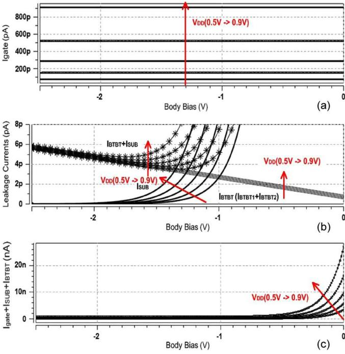
Fig. 4. Standby ( $V_{GS} = 0$  V) leakage currents of a 32-nm n-MOSFET with  $t_{ox} = 0.9$  nm and  $W/L = 128$  nm/32 nm as a function of body bias voltage and supply voltage: (a)  $I_{gate}$ . (b)  $I_{SUB}$ ,  $I_{BTBT}$ , and  $I_{BTBT} + I_{SUB}$ . (c) Total Leakage current =  $I_{BTBT} + I_{SUB} + I_{gate}$ .
