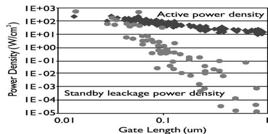
Fig. 2. Power density trends for the active power and the standby leakage power with CMOS (channel length) scaling
