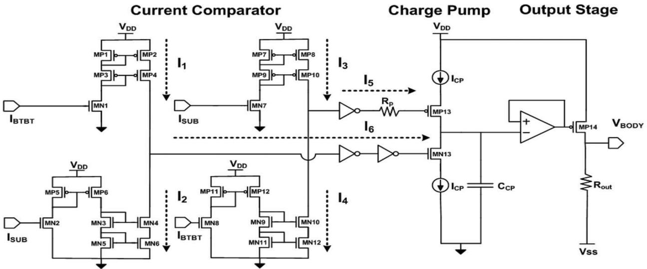
Fig. 12. Schematic of the proposed  $V_{Body}$  control system.
