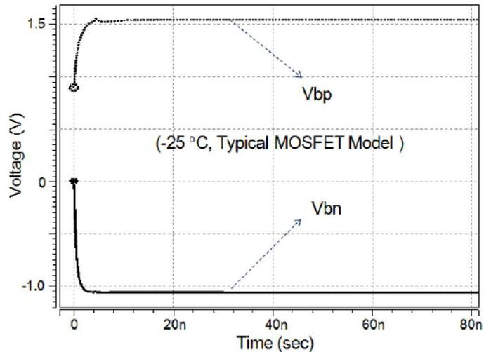
Fig. 11. Body bias voltage generated in the optimal body bias voltage controller.
