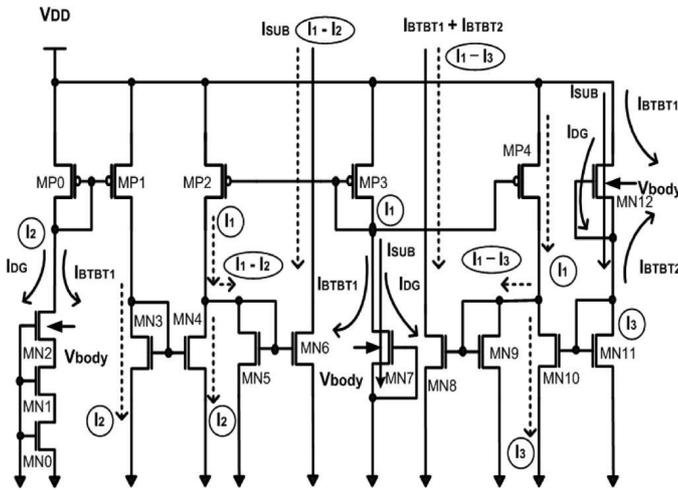
Fig. 10. Proposed leakage monitoring circuit for n-MOSFETs.
