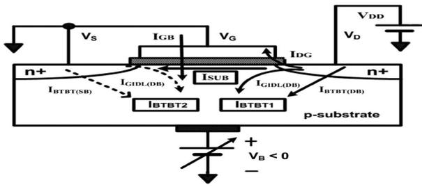
Fig. 3. Standby leakage current components under reverse body bias.
