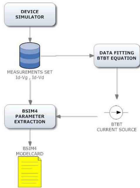
Fig. 4: BTBT source added to BSIM4 DC equivalent circuit
