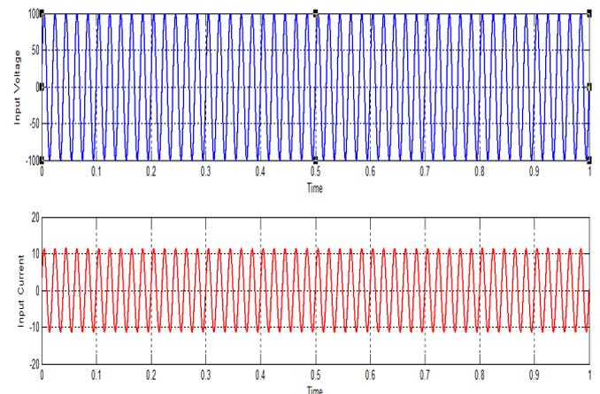
Fig 5 Waveforms of Input Voltage & current.
