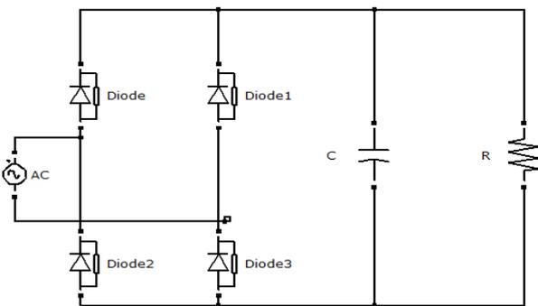
Fig.1. AC-DC Converter (Rectifier)
