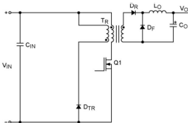
Fig.2. Forward Converter
