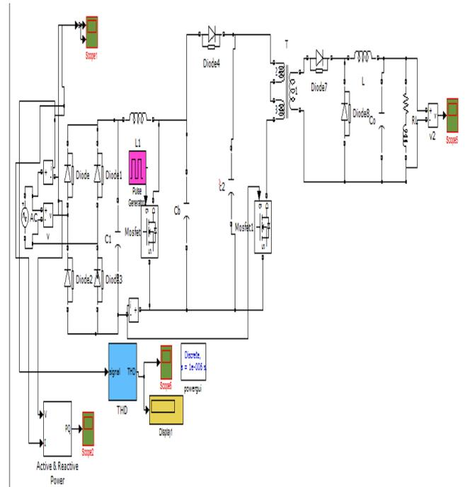
Fig.4: Simulink Model of Power factor correction with cascaded rectifier, boost converter and forward converter for RL load.
