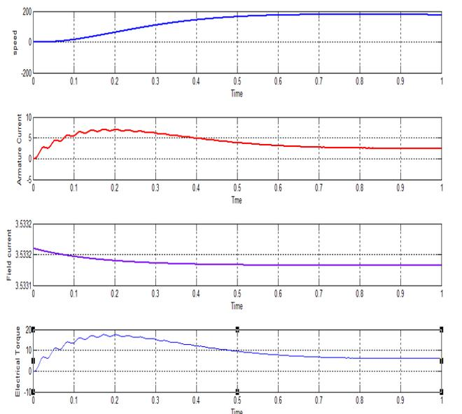
Fig.10: Waveform of speed, Armature Current, field Current, Torque of DC Motor 2.
