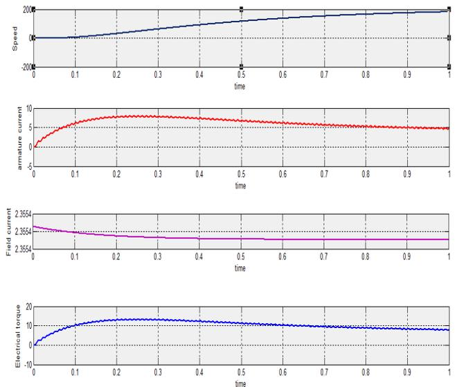
Fig. 9. Waveforms of speed, armature Current, Field Current and Torque of Dc motor 1.
