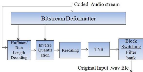
Figure 6: Low Complexity Advanced Audio Decoder
