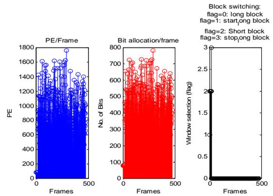
Figure 13: Plot of PE, bit allocation and bock switching decision per frame
