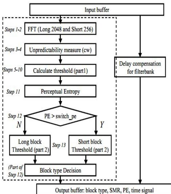
Figure 7 : Block diagram of PAM (ISO 13818-7) [15]
