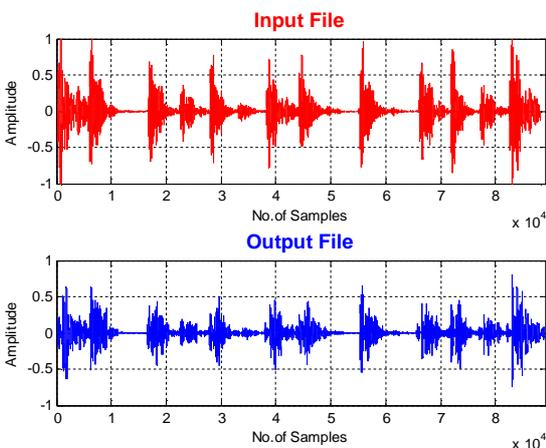
**Figure 14: Input (Original) and Output (Decoded) waves; File: drumsA.wav**
