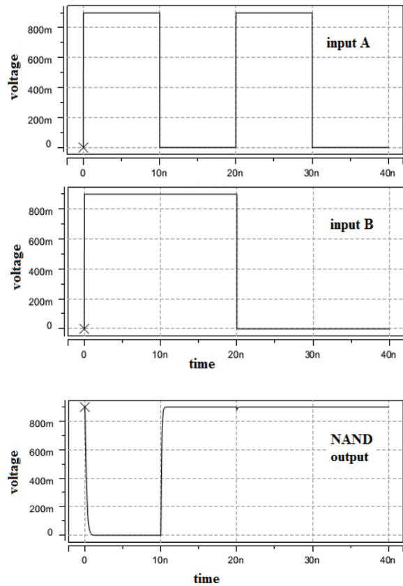
Fig 8: Structure of CNTFET NAND Gate and its behaviour
