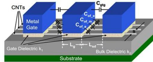
Fig.4: The 3-D structure of MOSFET like CNFETs with multiple channels
