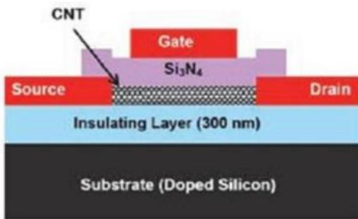
Fig.3:structure of CNTFET
