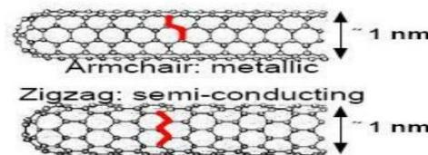
Fig.2: metallic and semiconducting CNT
