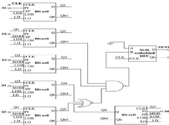
Fig.5. Asynchronous 6-bit S-counter.
