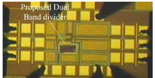
Fig.7. Die photograph of the proposed multiband divider.
