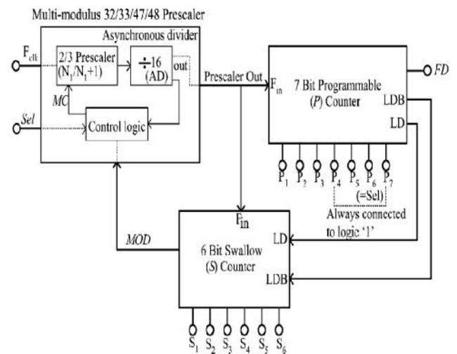
Fig.1. Proposed dynamic logic multiband flexible divider.
