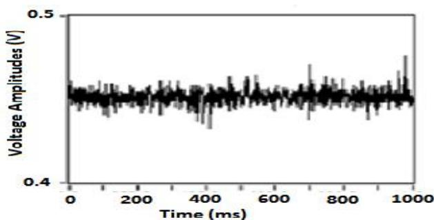
Fig. 3(a) Unfiltered detector voltage (V) obtained at labVIEW terminal versus time (ms).
