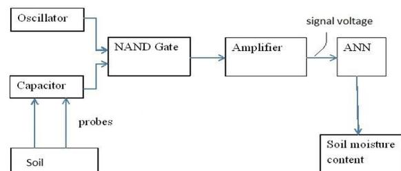
Figure1: Block diagram of soil moisture sensing technique
