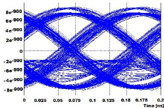
Fig. 4. Eye patterns of received signal at (a)  $\lambda=1545.80$  nm
