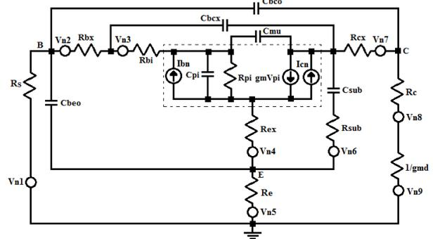
Figure 9: Electrical noise model representation of one side of Input Buffer
