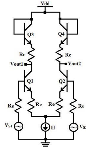
Figure 8: Circuit schematic of an Input Buffer
