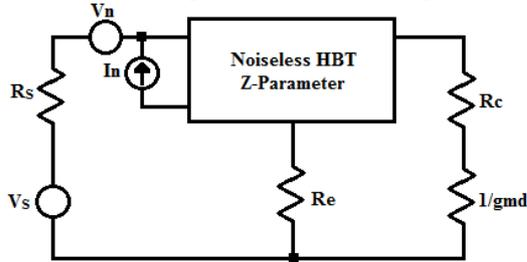
Figure 11: Series feedback amplifier with noise source
