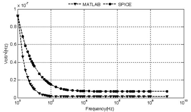
Figure 12: Reduction in input referred noise voltage after optimization
