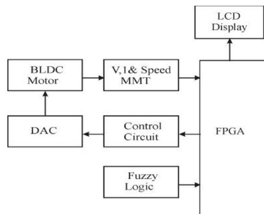
Figure 1. Block Diagram
