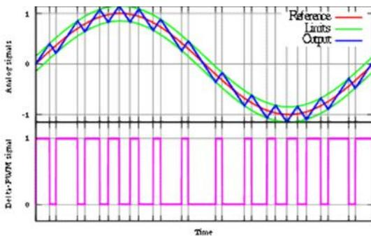
Figure 3.Principle of delta PWM.
