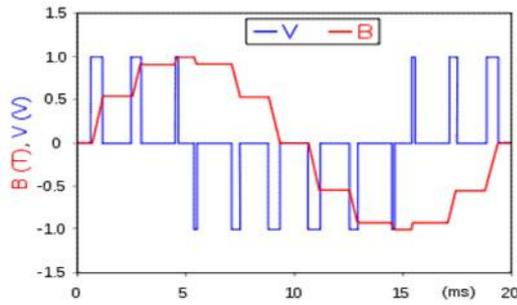
Figure 2.PWM in an AC Motor Drive
