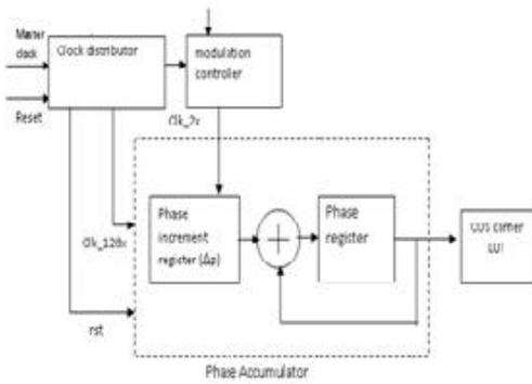
Figure 3 Direct Digital Synthesizer
