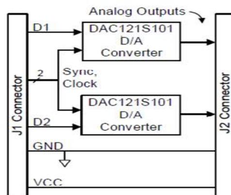
Figure 5 DAC Block Diagram
