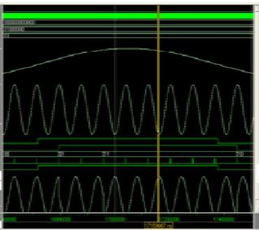
Figure 10 Simulation of QPSK
