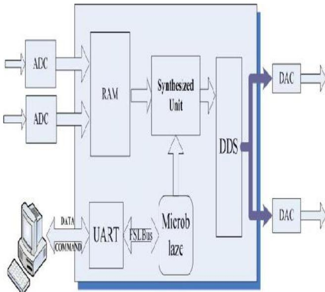
Figure1 processing module for FPGA
