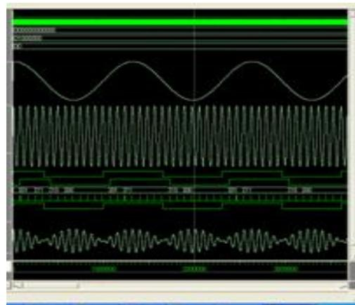
Figure 7 Simulation of AM
