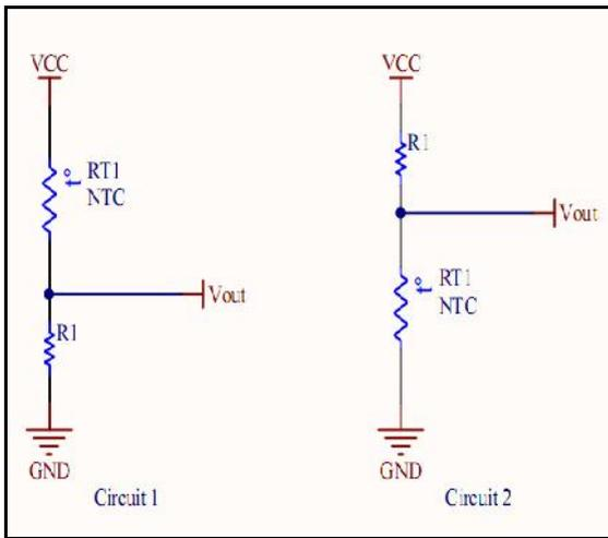
Fig. 8. Thermistor Circuit Diagram
