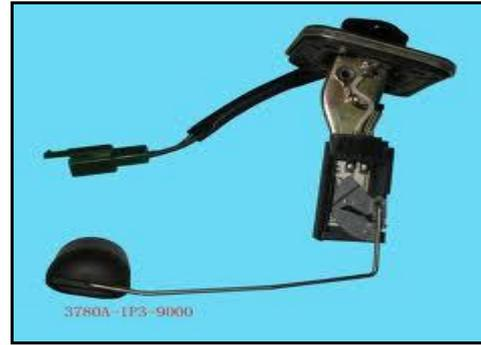
Fig. 9. Resistive fuel level sensor
