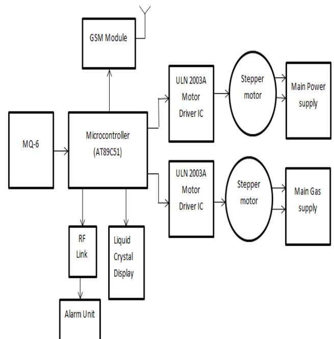
Fig. 1 Block diagram of gas leakage security system.
