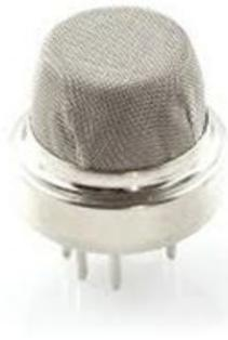
Fig. 2 MQ-6 gas sensor [5]
