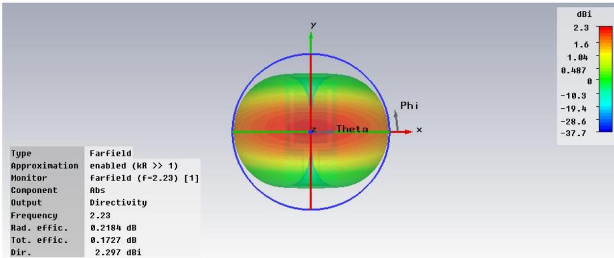
Fig. 4(a) 3-D Radiation pattern of Patch antenna showing directivity at 2.23 GHz
