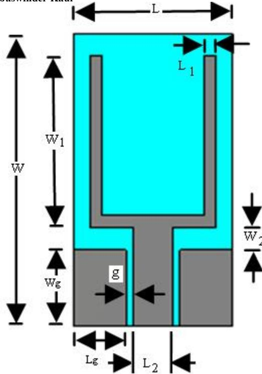
Fig. 1: Geometry view of proposed dual band antenna
