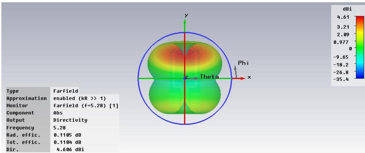
Fig. 4(b) 3-D Radiation Pattern of Patch antenna showing directivity at 5.28 GHz
