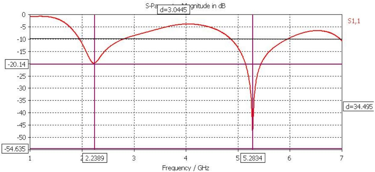
**Figure 2: Simulated Return Loss Curve**
