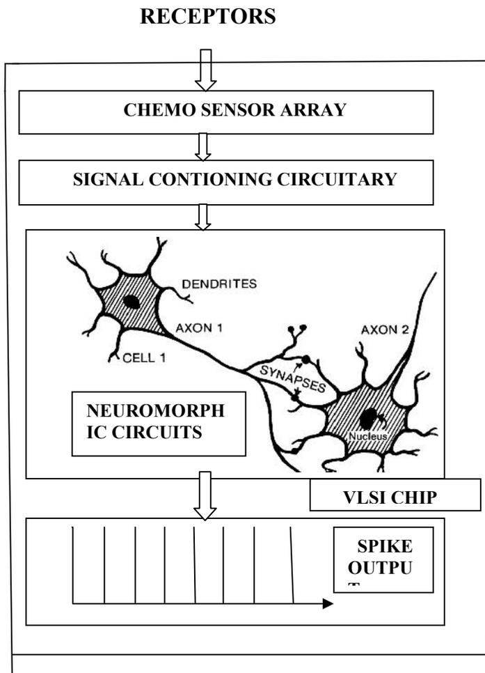
Fig.1.Sytem diagram .In this paper, receptors cells are realized by chemo gas sensors, where as signal conditioning circuitry receives the sensory signals from chemo sensors e array are digitally stored using analog to digital converter. neuromorphic circuits are integrated into a single chip.
