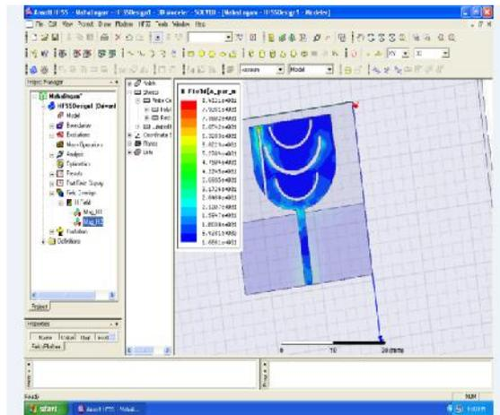
Fig 3.3 Current distribution at 4.5GHz
