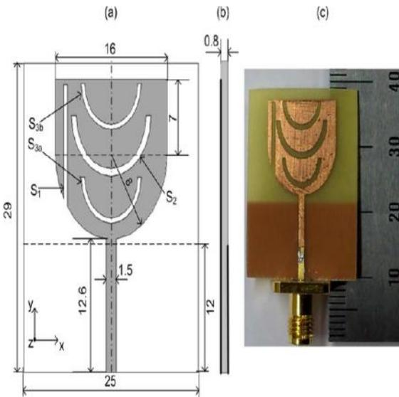
Fig 2.1 Dimensions of the antenna
