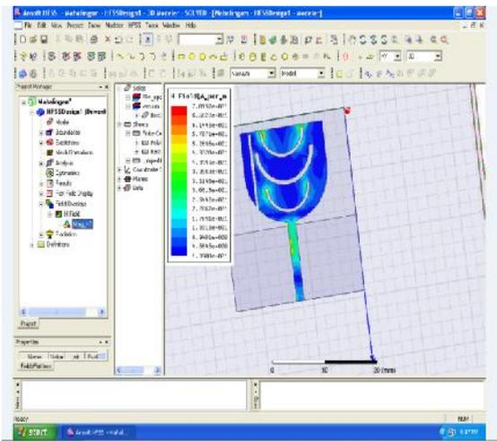
Fig 3.4 Current distribution at 7.5GHz
