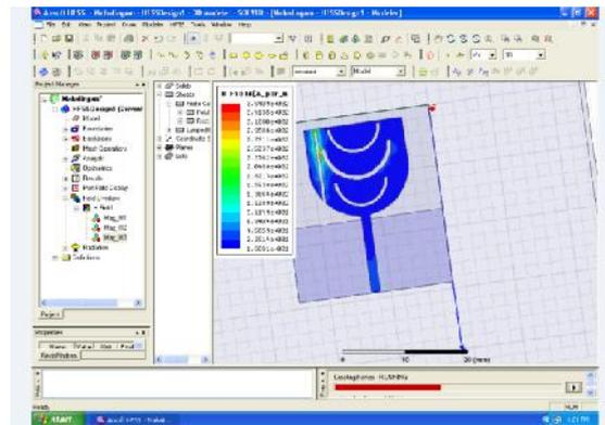
Fig 3.2 Current distribution at 3.5GHz
