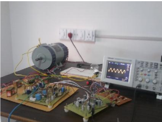
Fig. A4 Control and bridge rectifier circuits with motor load.
