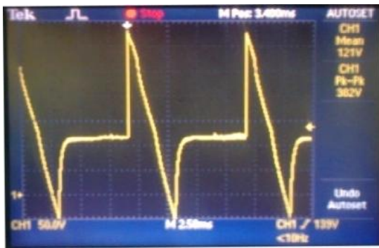
Fig. 17 (b) Experimental result for output of bridge rectifier for firing angle, \alpha=120^\circ .
