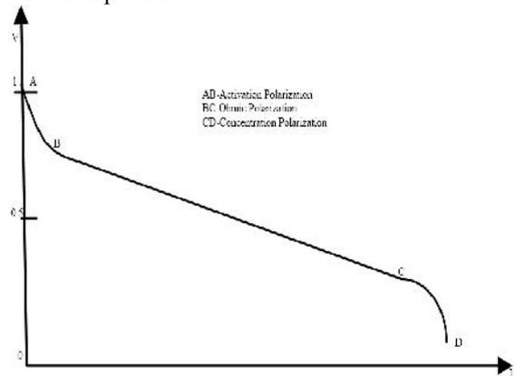
Fig. 3 V-I characteristic of a unit fuel cell
