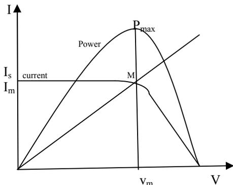
Fig. 2 Characteristics of a PV panel
