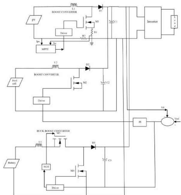
Fig. 6 Block diagram of a Hybrid Power System
