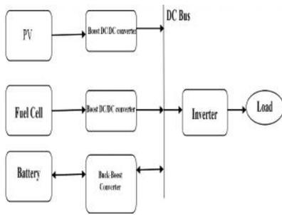
Fig. 1. Architecture of proposed hybrid power system
