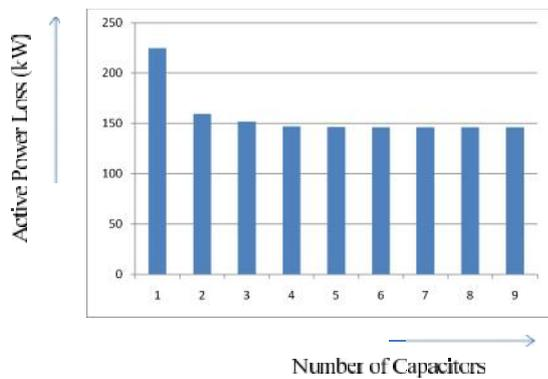
Fig. 1 Reduction in active power loss by capacitive compensation
