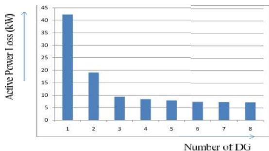
Fig. 2 Reduction in active power loss by DG placement
