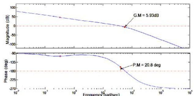
Fig. 5 Frequency response for Singular frequency based tuning
