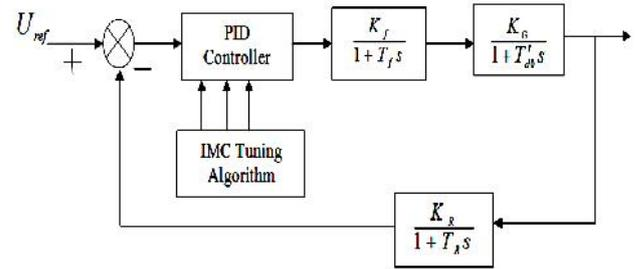
Fig. 1 Transfer Function of Generator Excitation System.
