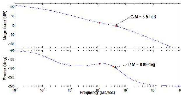
Fig. 6 Frequency response for Ziegler-Nichols closed loop based tuning
