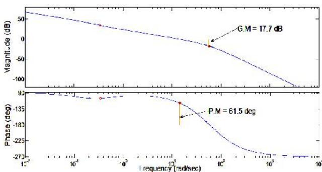
Fig. 7 Frequency response for IMC based design tuning
