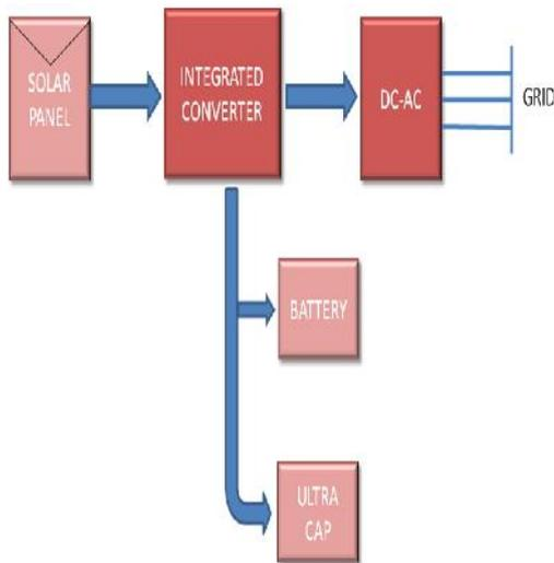
Fig 6.1 Block diagram of SPGS with Integrated Converter
