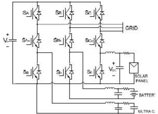
Fig 6.2 Circuit diagram of SPGS with Integrated Converter
