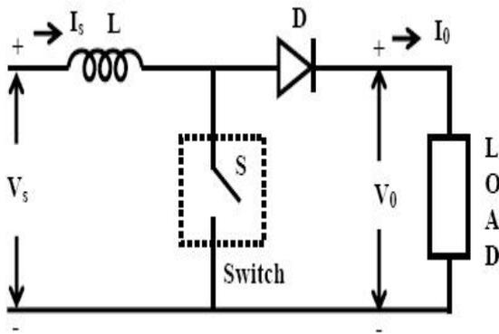
Fig 3.1(a) Boost converter (DC-DC)
