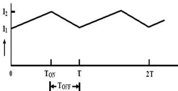
Fig 3.1(b) Waveforms of source current ( $i_s$ )
