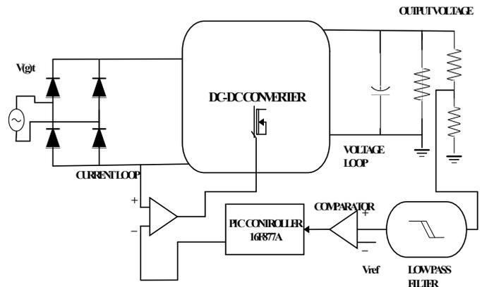
**Fig 2 : circuit diagram of power factor correctors**
