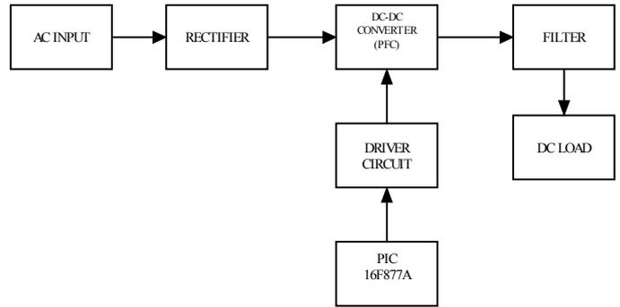
**Fig 1: block diagram of power factor correctors**
