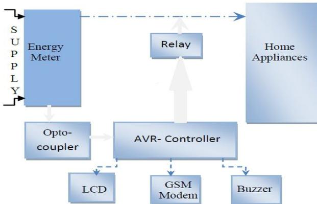
Fig. 1 Building Blocks of GSM Based Prepaid Energy Meter
