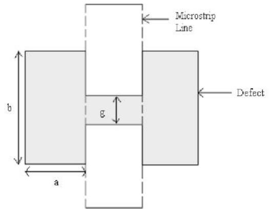
Fig 7. Dumb-bell Shaped DGS
