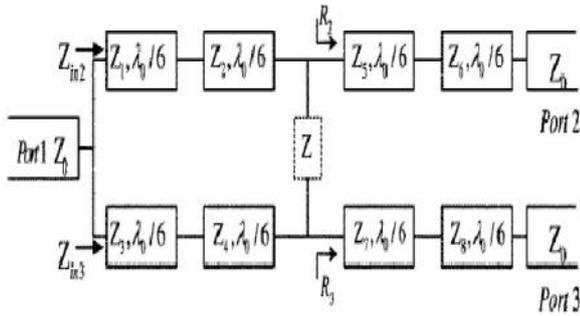
Fig 5. Dual frequency Wilkinson Unequal Power Divider for a Frequency and Its First Harmonic
