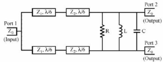
Fig 3. Dual frequency Wilkinson Power Divider for a Frequency and Its First Harmonic
