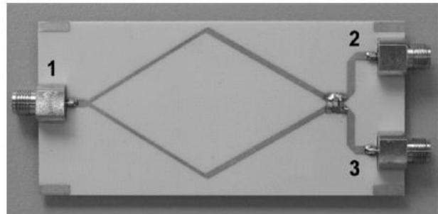
Fig 4. Dual frequency Wilkinson Power Divider
