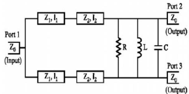
Fig 2. Dual frequency Wilkinson Power Divider
