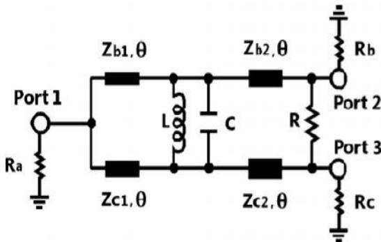
Fig 6. Parallel LC circuit at middle of dual frequency Wilkinson Power Divider
