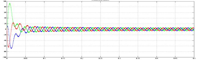
**Figure 9 Inverter Line currents**
