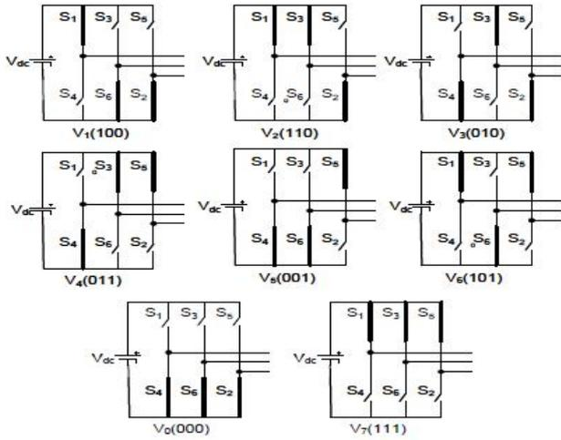
Figure 2 Switching States of SVPWM
