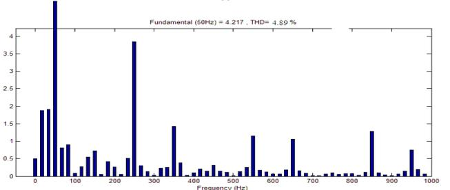
**Figure 14 Harmonic (FFT) Analysis of Line current**
