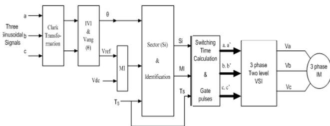
**Figure 7 Simulation Block Diag. of SVPWM Three level inverter with IM load**
