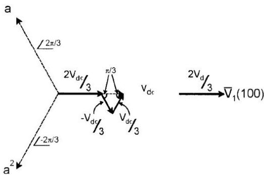
Figure 3 Construction of space vector V1 (100)
