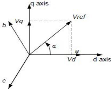
Figure 5 Voltage Space Vector and its d, q axis
