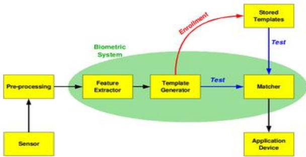
Figure: 1: The basic block diagram of a biometric system
