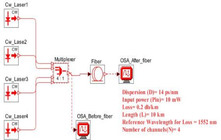
Figure 4. Layout for 4-channel WDM (with  $P_{IN}=10mW$ )
