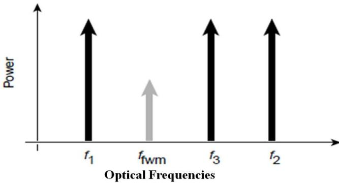
Figure 3. Four Wave Mixing
