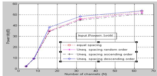
Figure 14. No. of Channels (N) Vs Power Tilt (dB) for  $P_{IN} = 1 \text{ mW}$
