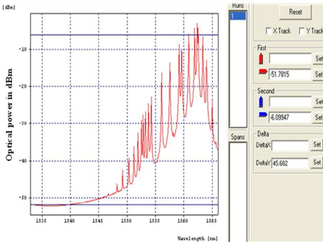
Figure 13. Optical Spectrum after the Fiber
