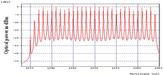
Figure 10. Optical Spectrum before the Fiber
