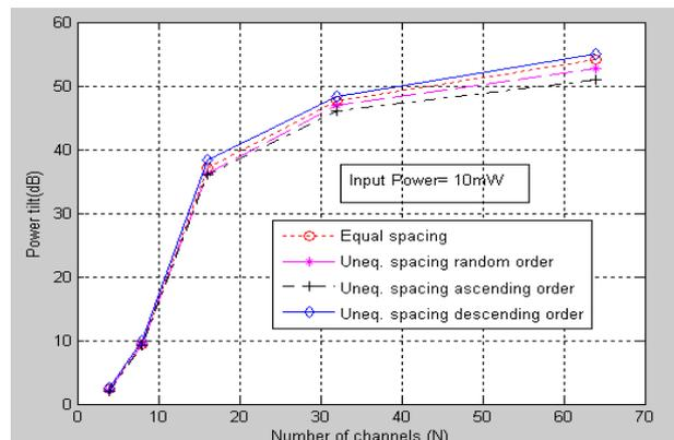
Figure 15. No. of Channels (N) Vs Power Tilt (dB) for  $P_{IN} = 10 \text{ mW}$
