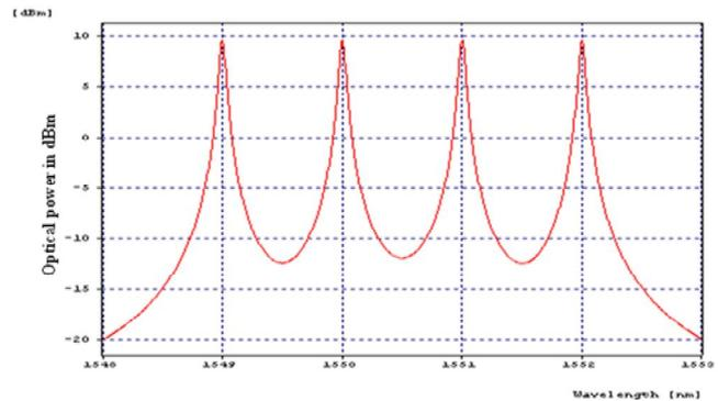
Figure 5. Optical Spectrum before the Fiber
