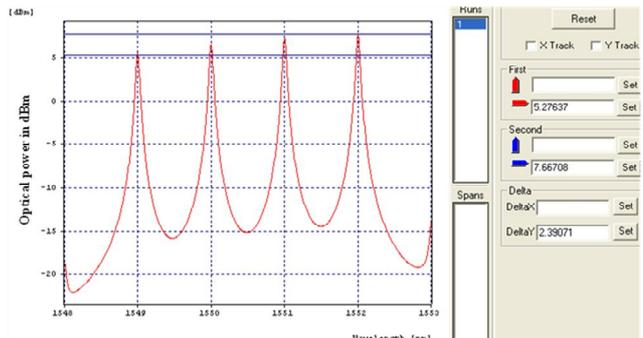
Figure 6. Optical Spectrum after the Fiber
