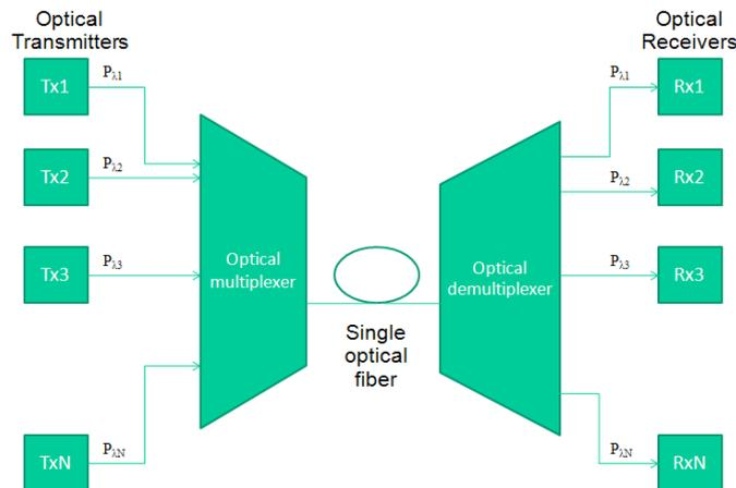
Figure 1. Dense Wavelength Division Multiplexing
