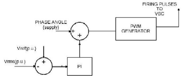
Fig.4. Block diagram of phase shift control
