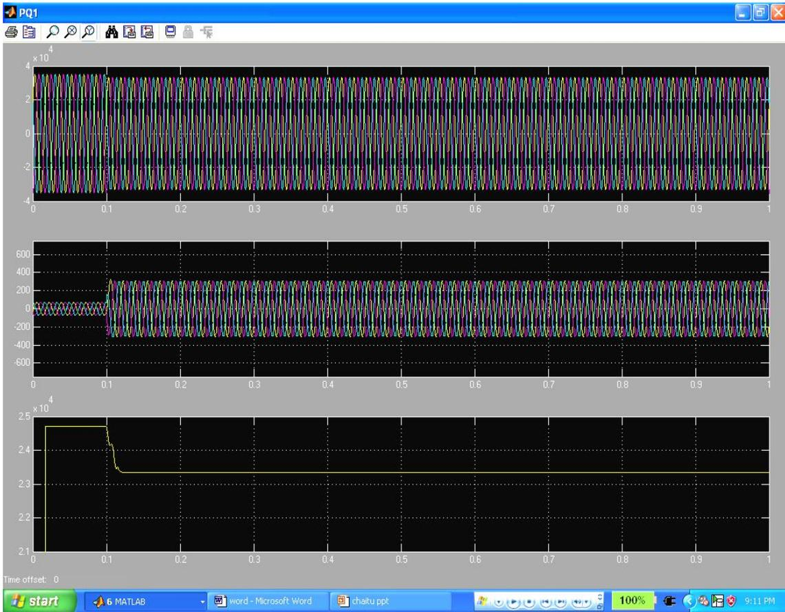
Fig.13..load voltage, load current & load voltage magnitude respectively with Inductive load in the uncompensated line
