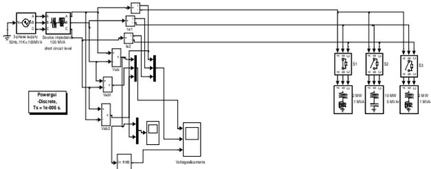
Fig.15. Simulink model of uncompensated lines with capacitive & inductive load
