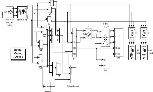
Fig.20. Simulink model of compensated lines with capacitive load
