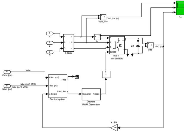
Fig.9. PWM based model of VSC implemented in SimPowerSystems.
