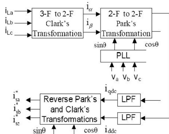
Fig.6. block diagram for synchronous frame theory
