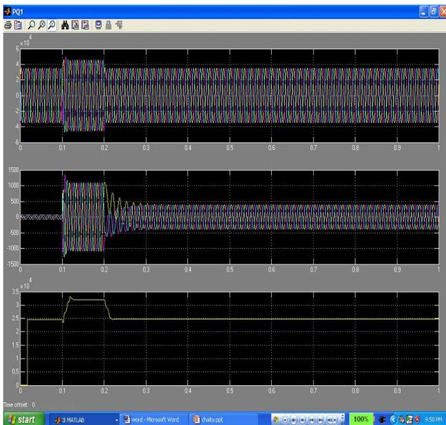
Fig.16. load voltage, load current & load voltage magnitude respectively with Capacitive & inductive load in the uncompensated line
