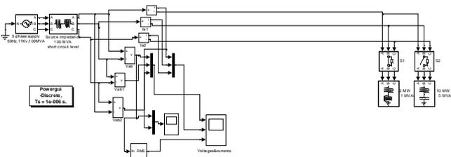
Fig.14 simulink model of uncompensated lines with capacitive load
