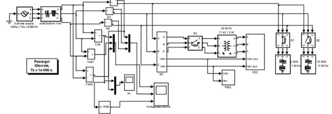
Fig.17. Simulink model of compensated lines with inductive load
