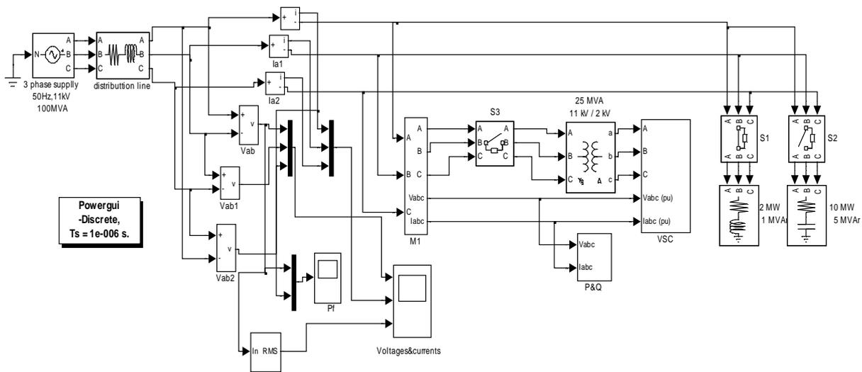
Fig.8. DSTATCOM connected to 11kV distribution system
