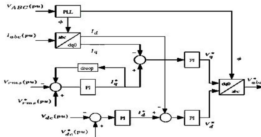
Fig.10 Voltage controller of DSTATCOM
