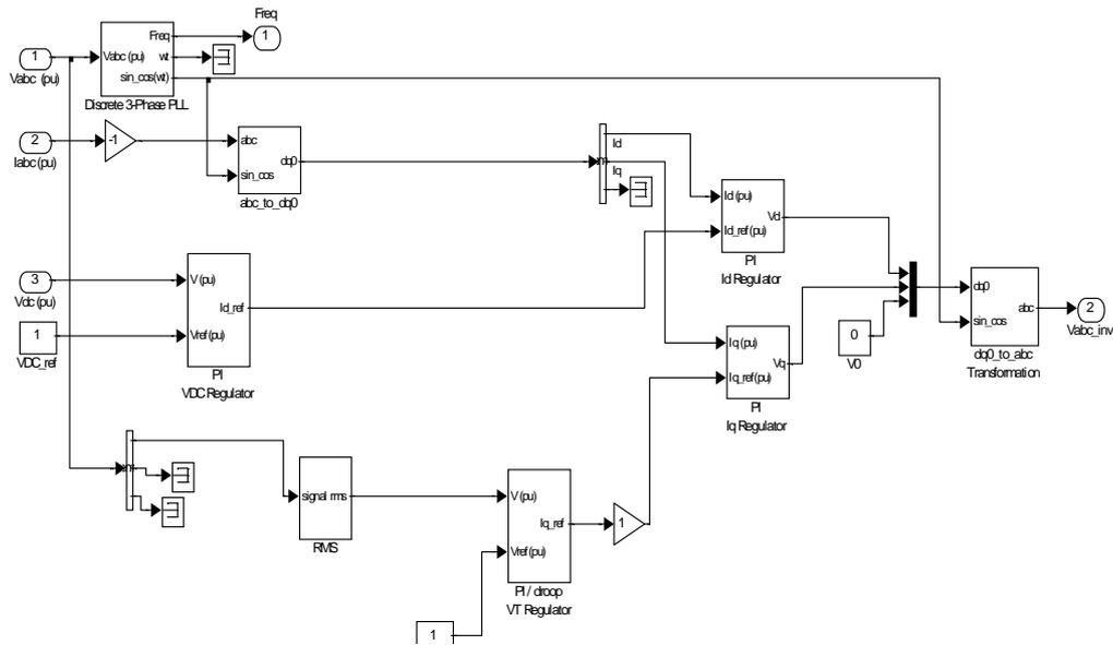
Fig.11.Voltage controller implemented in SimPowerSystems.
