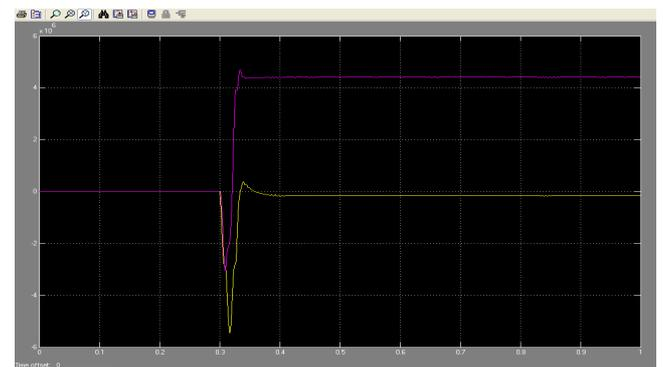
Fig.19. Reactive power of compensated lines with inductive load
