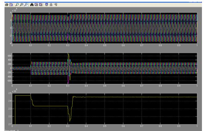
Fig.18. Load voltage, load current & load voltage magnitude respectively with Inductive load in the compensated line
