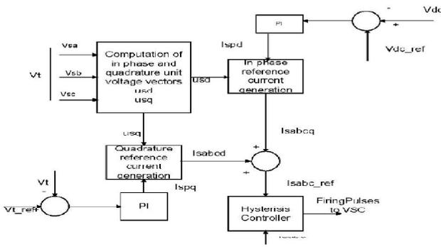
Fig. 7. Block diagram of regulation of bus and DC link voltage control
