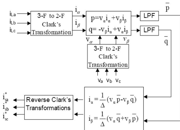
Fig.5. block diagram of decoupled theory based control of DSTATCOM
