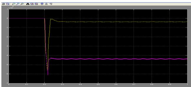
Fig.22. Reactive power of compensated lines with capacitive load
