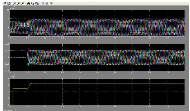
Fig.15. load voltage, load current & load voltage magnitude respectively with Capacitive load in the uncompensated line
