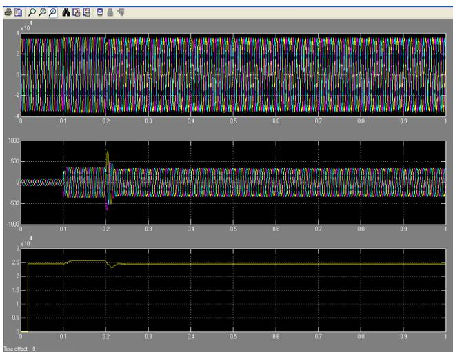
Fig.21. Load voltage, load current & load voltage magnitude respectively with Capacitive load in the compensated line
