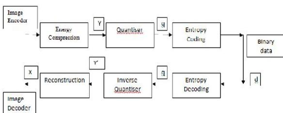
Fig1. Different steps of image compression and decompression
