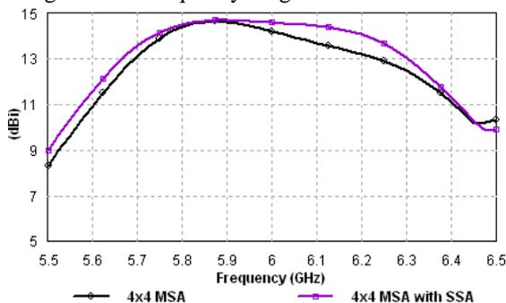
Fig.4 Total Field Gain Vs. Frequency
