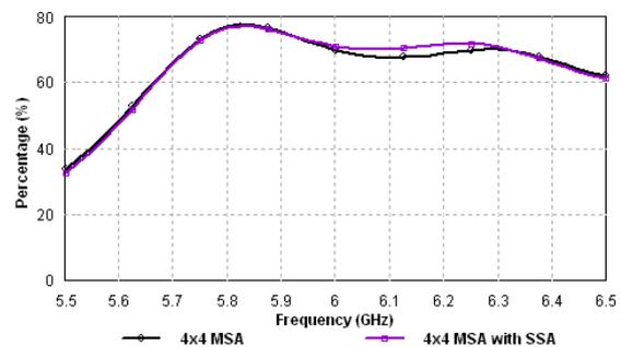
Fig.7 Antenna Efficiency Vs. Frequency
