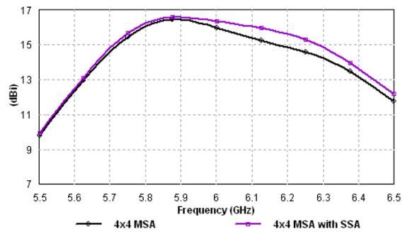
Fig. 5 Total Field Gain Vs. Frequency
