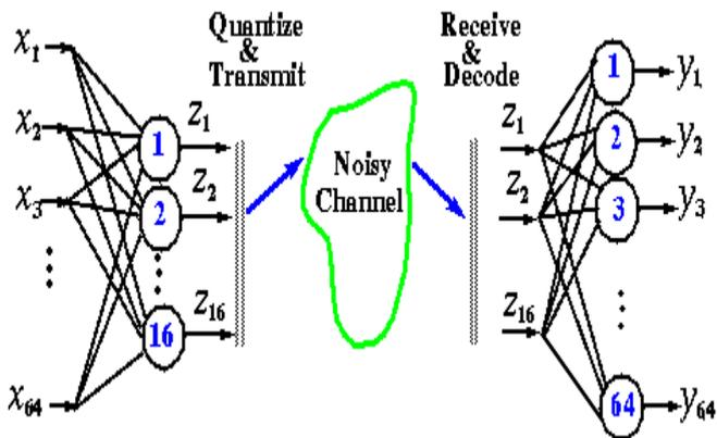
Figure 3.2 Image Compression Scheme using the Trained Neural Net
