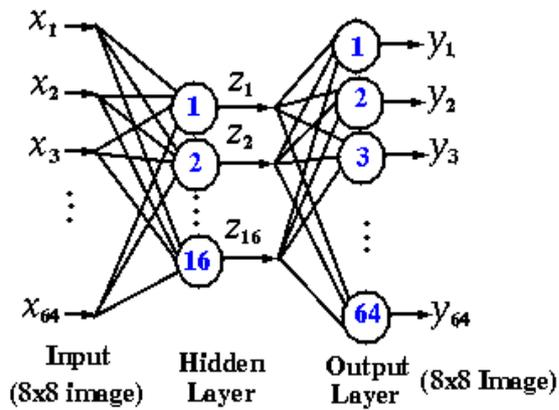
Figure 3.1 Bottleneck-type Neural Net Architecture for Image Compression
