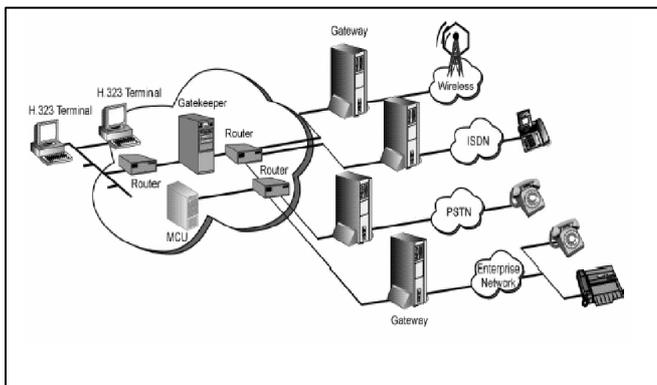
**Figure2. VoIP Network Components**
