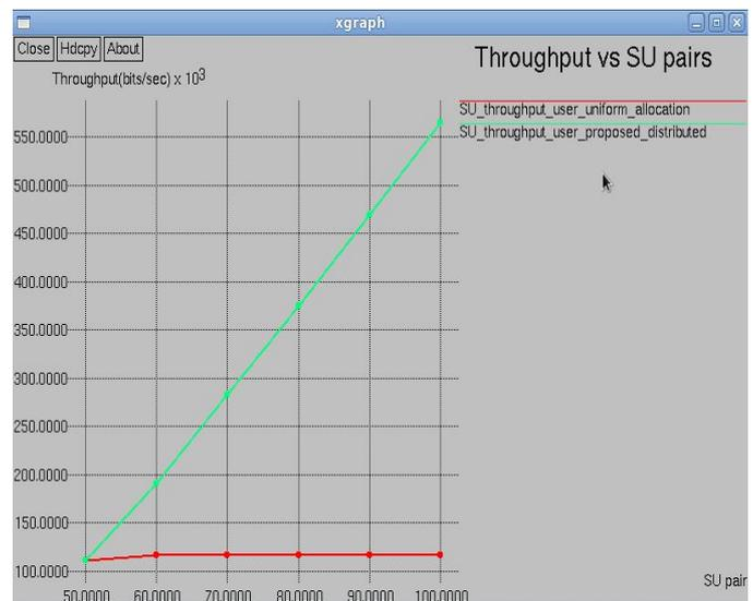
Fig. 3 Throughput versus SU pairs in Cognitive Radio Network
