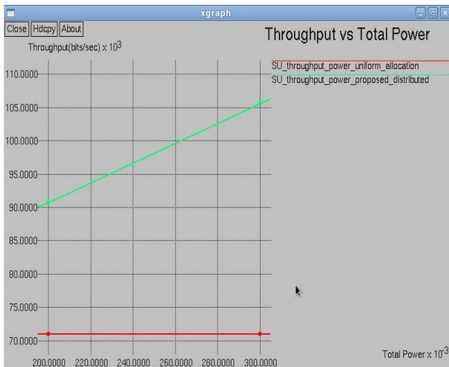
Fig. 5 Throughput versus Total Power using distributed scheme
