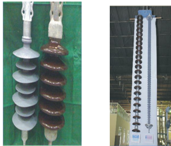
Fig.13 Traction and Long Rod Insulators
