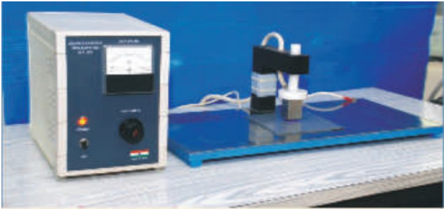
Fig.8 Hydrophobicity test setup
