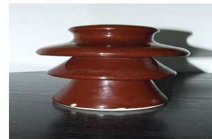
Fig.1. 10kV Porcelain Insulator
