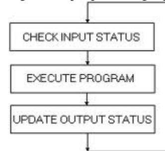
Fig.5. PLC scan process
