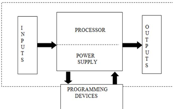
Fig.4. Block diagram of Programmable Logic Controller
