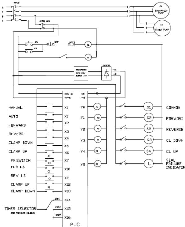
Fig.6. Electrical wiring diagram of Hydraulic Pressure Test Machine
