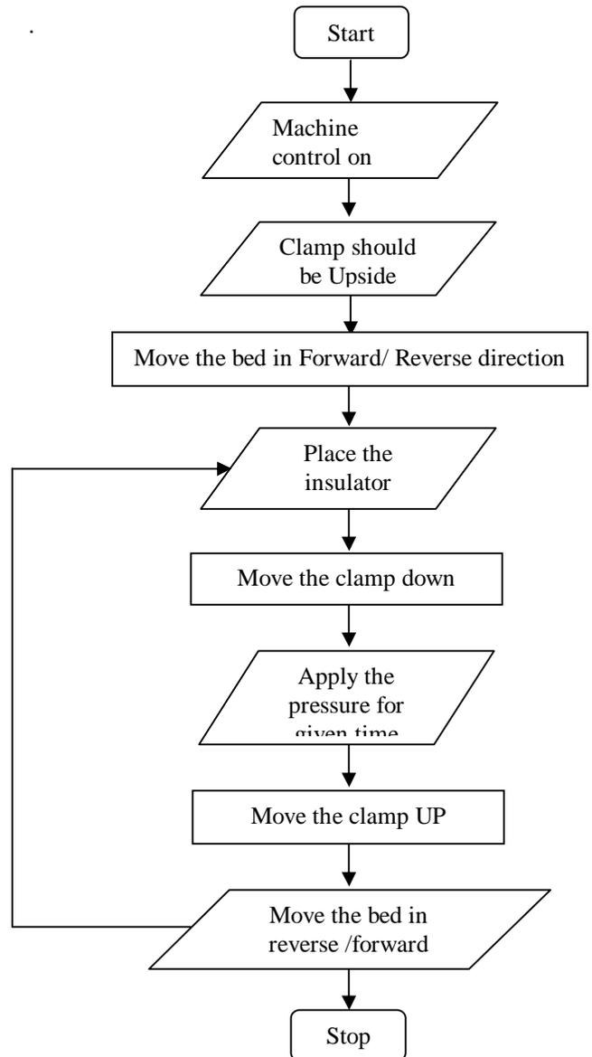
Fig.7. Flow chart of the working sequence of Hydraulic Pressure Test Machine
