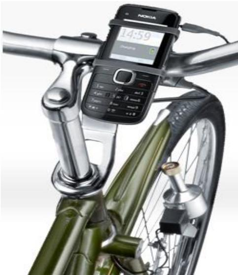
**Fig 7: Charging of a mobile using pedalling**
