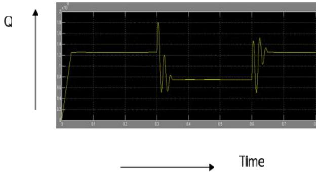
Fig. 11 Variation of Qline with Step Change of 50 MVar without Controller
