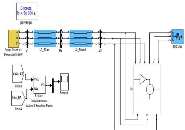
Fig. 6 Simulink Model of UPFC Connected Transmission Line
