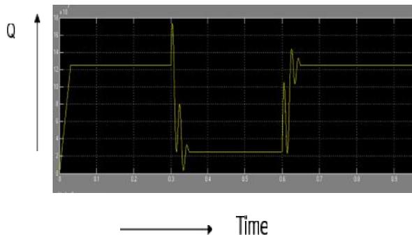
Fig. 9 Variation of Qline with step change of 100 MVA<sub>r</sub> without controller
