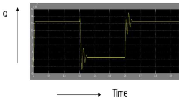
Fig 10 Variation of Qline with step change of 100 MVA<sub>r</sub> with controller
