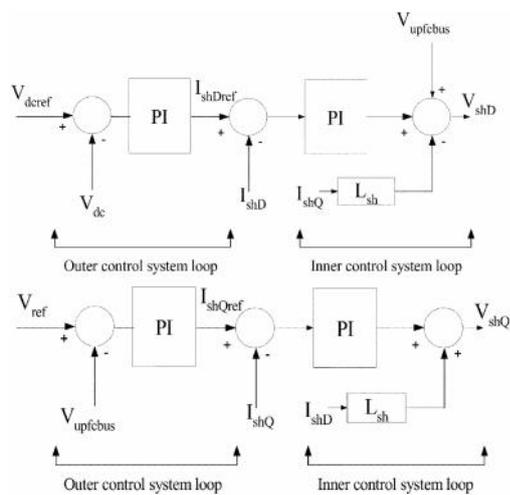
Fig. 1 De-Coupled D-Q axis Shunt Converter Control System.
