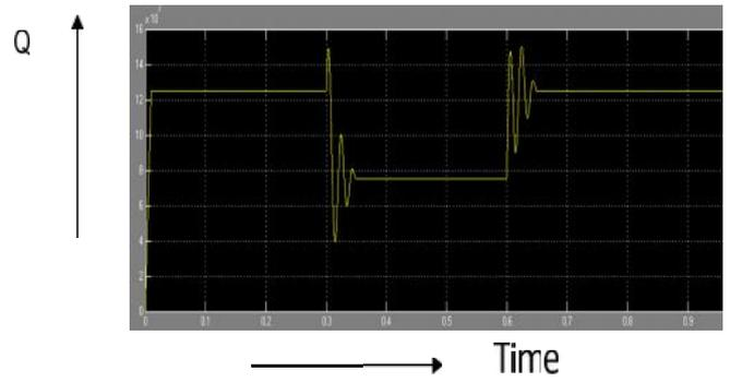
Fig 8 Variation of Qline with step change of 50 MVA<sub>r</sub> with controller
