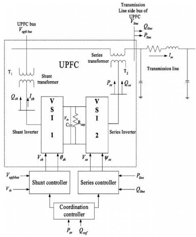
Fig. 3: UPFC Connected to a Transmission Line.
