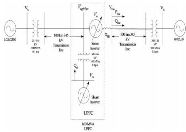
Fig. 5 Power system with UPFC.
