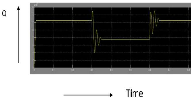
Fig. 12 Variation of Qline with Step Change of 50 MVar with Controller
