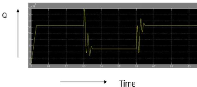
Fig. 7 Variation of Qline with step change of 50 MVA<sub>r</sub> without controller
