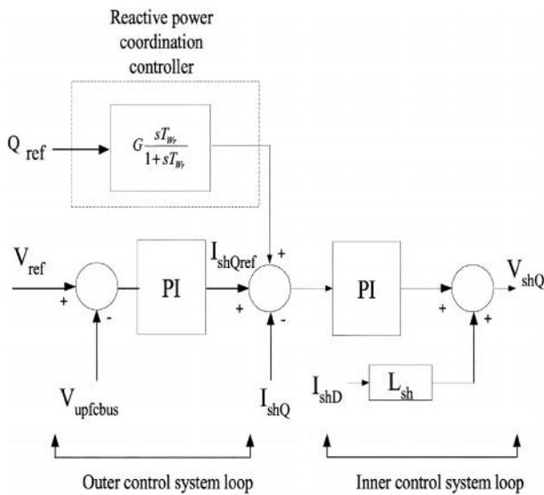
Fig. 4. Shunt Converter Q-Axis Controller with Reactive Power Coordination Controller.
