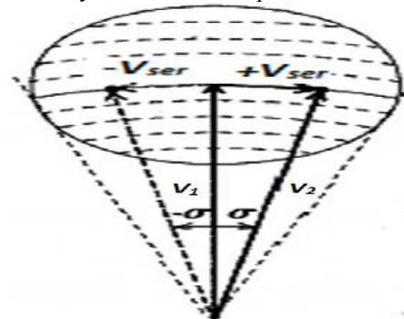
Fig.8UPFC working as a phase angle regulator/shifter [11]
