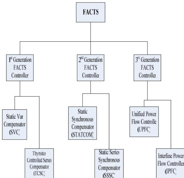
Fig.1 Block Diagram of FACTS Controllers [8].
