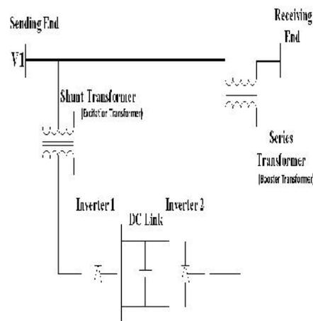
Fig. 5 Schematic diagram of a UPFC system [9]
