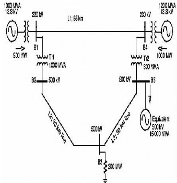
system. Fig 11 One line diagram of 500/230 kV Transmission System [12]
