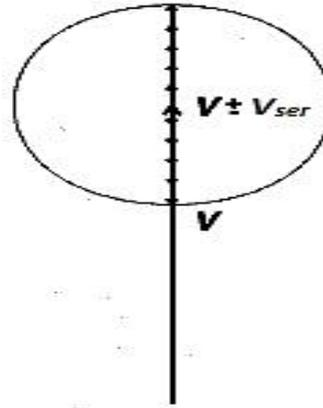
Fig.7 UPFC working as a voltage regulator [11]
