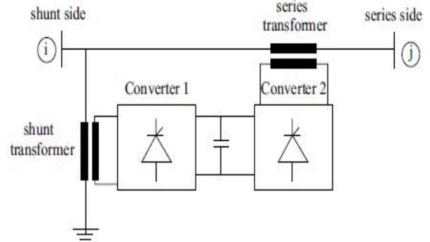
Fig.2 Unified Power Flow Controller (UPFC) [8].
