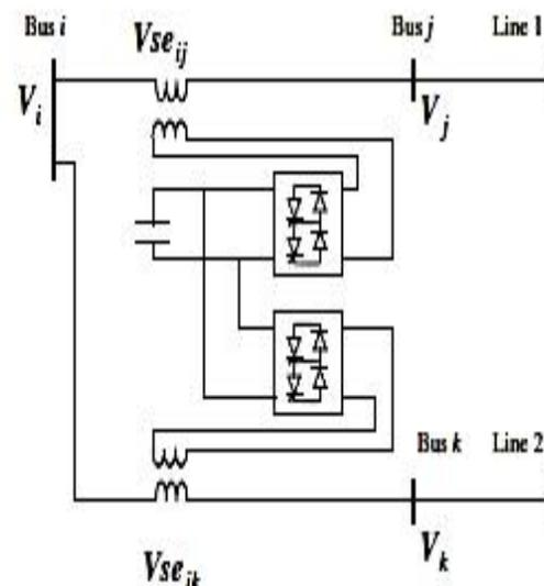
Fig. 3 Interline Power Flow Controller [9]
