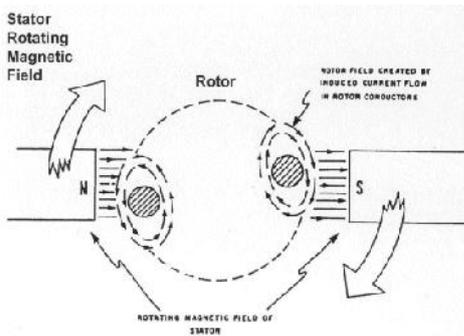
Figure 1: Operating principle of Induction motor
