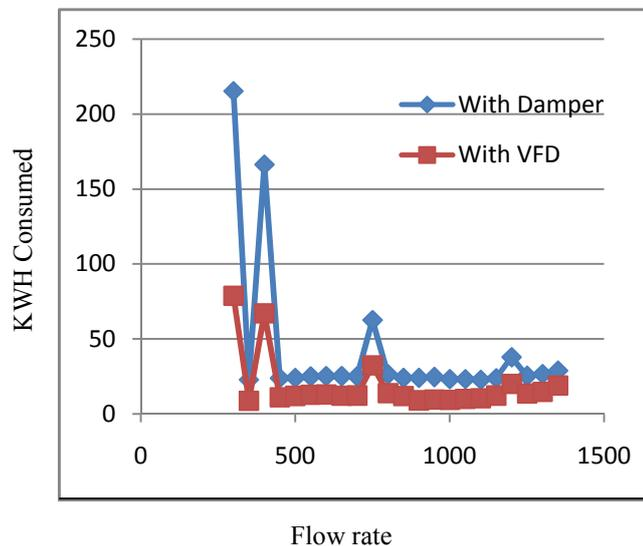
Figure 7: The Comparison of KWH Consumed When Damper and VFD are Used
