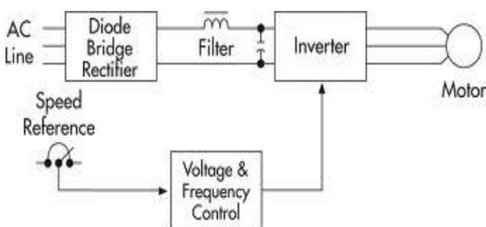
Figure 2: Electronic scheme for V/f control
