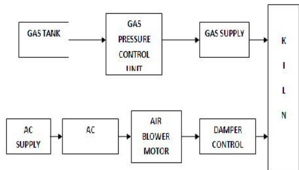
Figure 3: Block Diagram of treatment process
