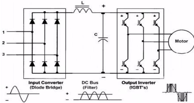
Figure 5: Circuit Diagram of Variable Frequency Drive
