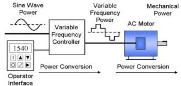
Figure 4: Variable frequency drive system
