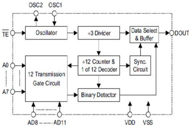
Figure 2.3: Block diagram of HT12E
