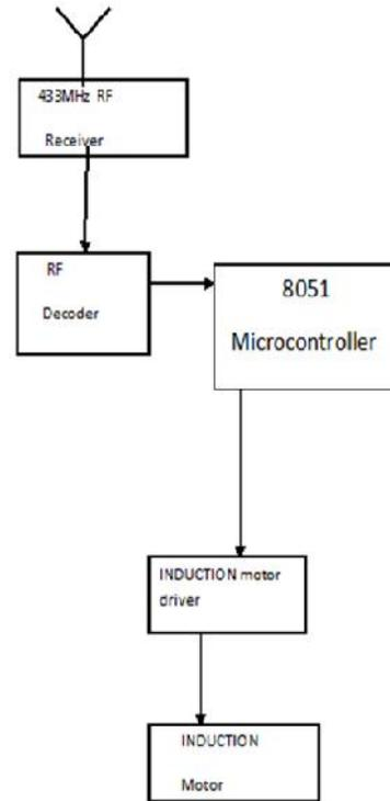
Figure 2.4: Block diagram of Receiver section
