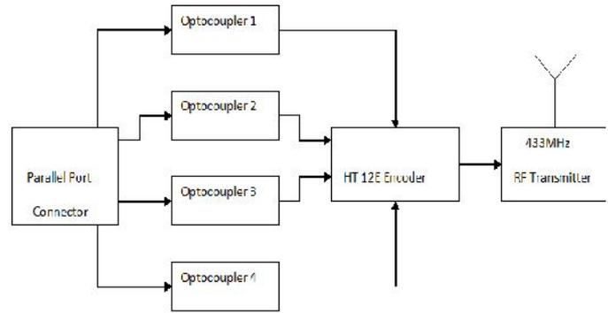
Figure 2.1 Transmitter section block diagram
